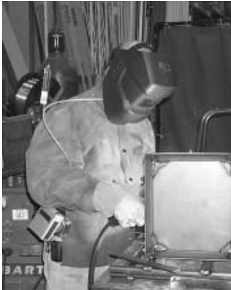
According to OSHA, if the employee is wearing a welding helmet and either no respirator or a negative-pressure respirator, sampling should be performed inside the helmet and outside any respirator.
