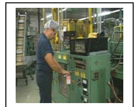
Verify Machine is in Safe Condition
