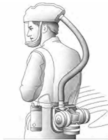
Loose-Fitting Powered Air-Purifying Respirator (PAPR) APF=25
